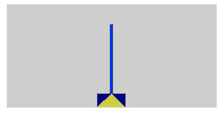
The rod initially has a mass of 0.21kg and a length of 0.61m and is stabilized via LQR control. The Appendix explains both the equations of motion for the system and the design of the LQR controller.
