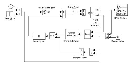
Tunable Variables are Matrix gain, K, and Feedforward gain, FF.
